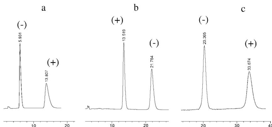
**Figure 2.** Chromatograms for chiral resolutions at room temperature. (a) Diclofop-methyl, 2% isobutanol, 230 nm, and 1.0 mL min<sup>-1</sup>; (b) ethofumesate, 5% isobutanol, 230 nm, and 1.0 mL min<sup>-1</sup>; and (c) benalaxyl, 2% butanol, 230 nm, and 1.0 mL min<sup>-1</sup>.
